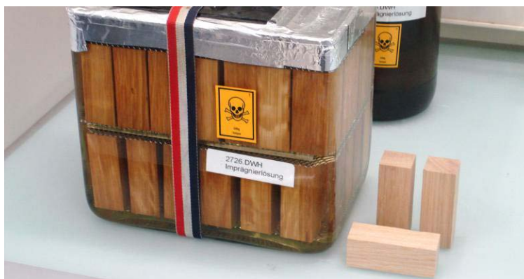
Figure 1 – Contamination of oak wood specimens in a glass container and storage of the contaminated pesticides under a laboratory hood
