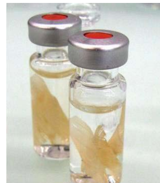
Figure 5 - Wood tissue sections placed in GC vials for pesticide extraction
